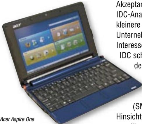
**Acer Aspire One A150L:** 8,9-Zoll WSVGA-Display, Intel Atom N270, 1,6 GHz, 1 GB RAM, 120 GB Samsung HDD, 3x USB 2.0, Mikrofon, SD Cardreader, 5-in-1 Cardreader, Crystal Eye Webcam, Wireless LAN 802.11b/g
